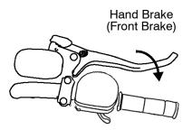
**WARNING!** Operating the ATV with a spongy brake lever can result in loss of braking, which could cause an accident. Never operate the ATV with a spongy-feeling brake lever. Always contact your dealer for service before operating the vehicle.
